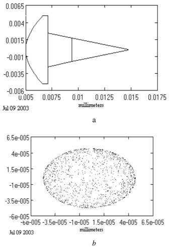
Fig. 1. Preliminary ray-trace analysis for a spherical micro-lens
