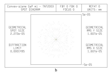
Fig. 2. Micro-lens with aspherical frontal surface
